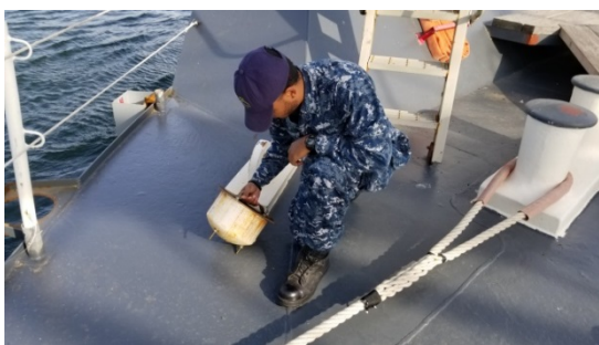
Fig. 8: Sailor Changes Stormwater filter
