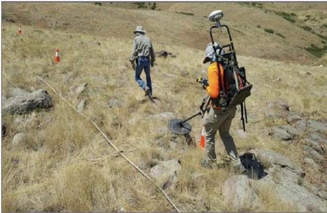
Field crews use the “Parsons Digital Mapper.” The hand-held digital geophysical mapping (DGM) device allowed technicians to perform DGM surveys in rugged terrain and with high magnetic interference. Rocky terrain and slopes are representative of the site.
