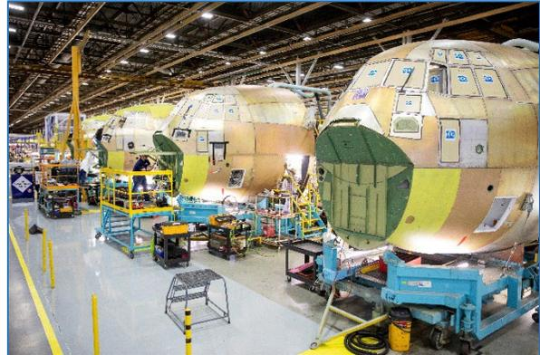
C-130J Forward Fuselage Section Assembly on the Government Owned, Contractor Operated Air Force Plant 6 Production Line in Marietta, GA
