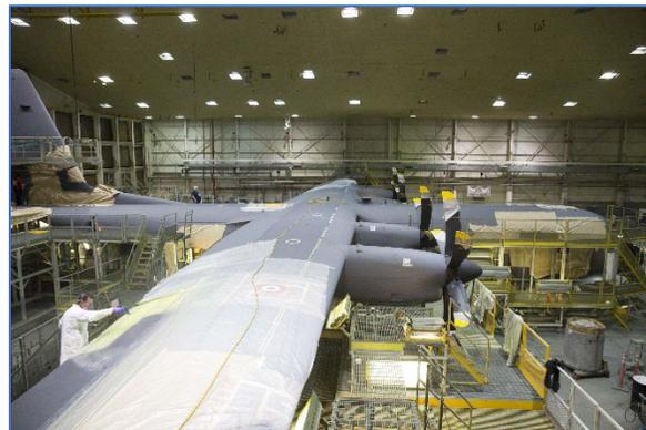
C-130J in the Paint Crib where the new Solvent Borne Non-Chrome Primer is applied, and Primer Reactivation Solvent is used as needed.
