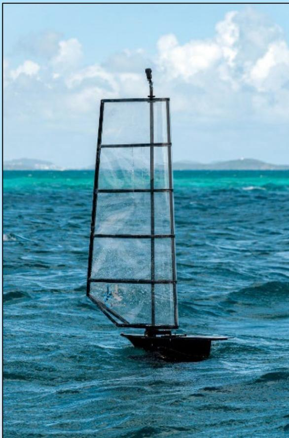
Figure 9. SubSeaSail, an autonomous semi-submersible capable of collecting critical scientific data, being field-tested in a Vieques bay containing thousands of munitions on and beneath the seafloor.
