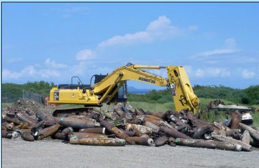
Figure 7. Inert munitions, including bombs up to 2,000 pounds, awaiting dismantling by the water jet, a system of high-pressure water and abrasive material that can cut munitions into manageable pieces for recycling and beneficial reuse.
