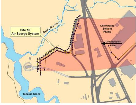
During 2002, O&M of the Site 16 Air Sparge System was contracted to a small business at a savings of more than \$21,000. The Air Station implemented air sparging at Site 16 as an interim measure to prevent groundwater contaminants from migrating to the environmentally sensitive Sandy Branch and Slocum Creek.
