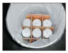
DNSC took measures to provide redundant protection for the mercury by over-packing the 76 pound flasks in 30-gallon sealed drums.
