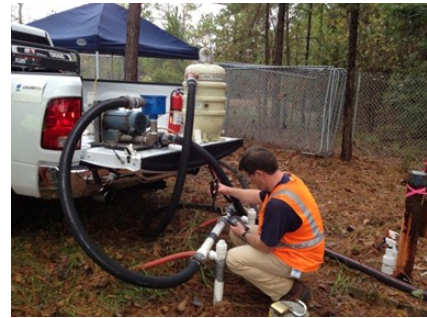
A remediation technology study is being conducted (pictured here) to evaluate potential groundwater treatment alternatives for selection of a final remedy. The study resulted in a reduction of concentrations to below detection limits within one month of start-up.
