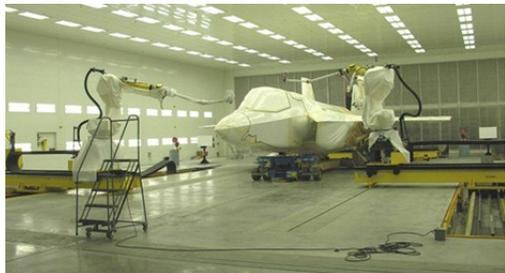
*Pictured here is a robotic painting work cell. A new lightweight coating system eliminates one layer of paint from the traditional system resulting in an overall aircraft weight reduction and over 50% reduction in the paint/pain-removal waste stream.*
