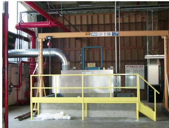
The Environmental Affairs Department recognized this concern and commissioned a study to evaluate less toxic paint strippers that still met MILSPEC standards. The results of this study allowed for the procurement of a Ramco AJA Kleen System with F0606 solvent for the squadron to replace the antiquated methylene chloride dip tank. Besides the clear benefit of elimination of methylene chloride and phenol, other benefits were recognized.
