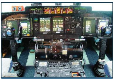
Shown above is the cockpit of the upgraded C-5M Super Galaxy. This aircraft includes the Avionics Modernization Program (AMP) upgrades. The CMC/Wx Radar Modification program upgrades will interface and be presented on the new digital readouts making the workload easier for pilots and crew alike and will provide much more real-time data than previous analog equipment.
