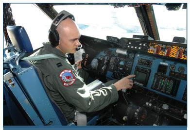
Pictured here, Capt. David Elkins, 22nd Airlift Squadron C-5 aircraft commander, examines the weather radar during a pre-flight check. This picture was taken in preparation of the Crisis Look 07-02 deployment exercise held on Travis Air Force Base, California. Within the cockpit can be seen the original, pre-CMC/Wx Radar Modification and pre-Avionics Modernization Program upgrades to the display equipment.
