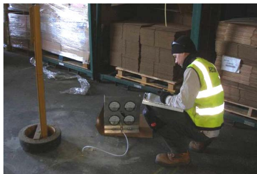
Figure 5: Scientists monitor vapor pressure inside installation facilities
