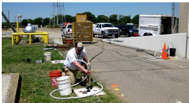
Figure 4: Scientist inject edible oil into the subsurface through monitoring wells to promote bioremediation
