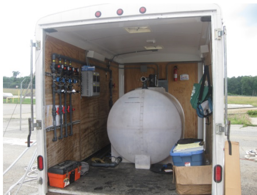
Figure 1: Trailer used for mixing and injection of Emulsified Vegetable Oil
