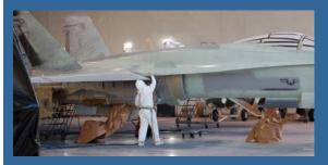
Figure 7: F/A-18 Being Painted for the Advanced Non-Chromate Primers & Coatings Project
