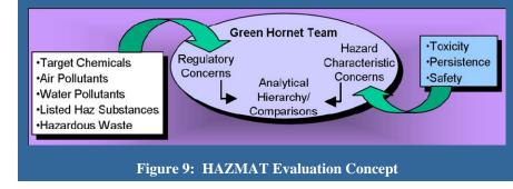
identified HAZMAT are validated against those materials approved on the Aviation and Shipboard HMLs. If a material is not on these lists, then either an alternative is identified or PMA265 works to have that
