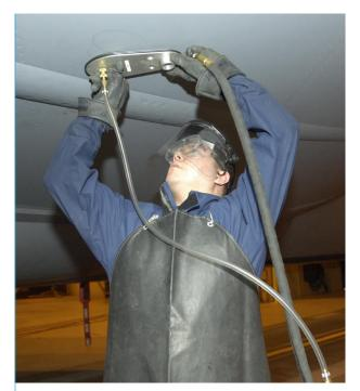
The new "sealvac" bowser unit is used to empty fuel cells and tanks prior to inspection and repair. The unit uses a special adapter plate which essentially eliminates JP-8 fuel spills. Reduced health exposure and reduced safety risks have also been realized.
