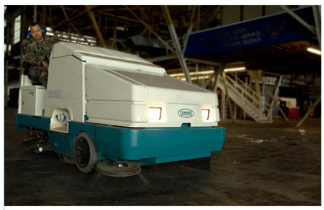
A recently purchase wet/dry floor sweeper is a big improvement over the older wet floor sweeper. Using a dry method for most floor cleaning operations with occasional wet "foam" cleaning, significantly less wastewater is now generated. The base estimates that this new unit will result in a 20,000 pound annual reduction in hazardous waste disposal.
