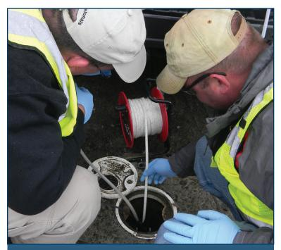
A synoptic groundwater elevation survey of 336 wells, along with water quality samples from 50 wells and a compilation of historical data, led to the development of a base-wide conceptual site model. The base-wide conceptual site model provides a holistic picture of Fairchild's hydrogeology. The base-wide conceptual site model also transforms conventional site-specific investigations to identify efficiencies to be gained and fine-tune site closure exit strategies.
