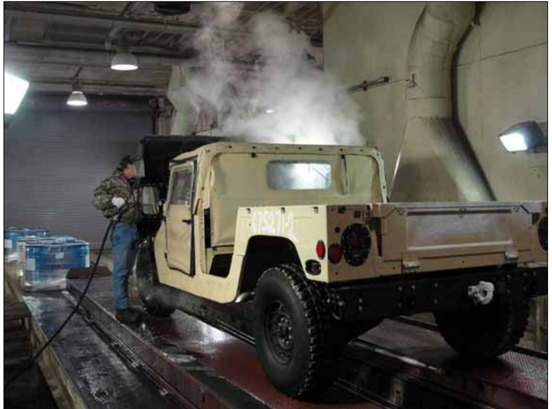
An employee is shown cleaning a vehicle with a high-pressure closed looped system. This system conserves water and minimizes discharge to the industrial wastewater plant.
