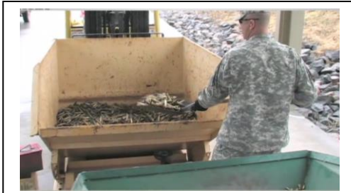
1SG Chad Turner is shown feeding recycled brass into the safety certification unit. Approximately 60 tons were treated and recycled in 2013. Ammunition Supply Point personnel assume responsibility for operating the unit.
