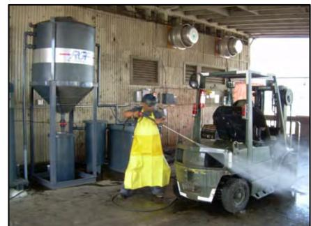
*Vehicle wash water recycling system in action.*
