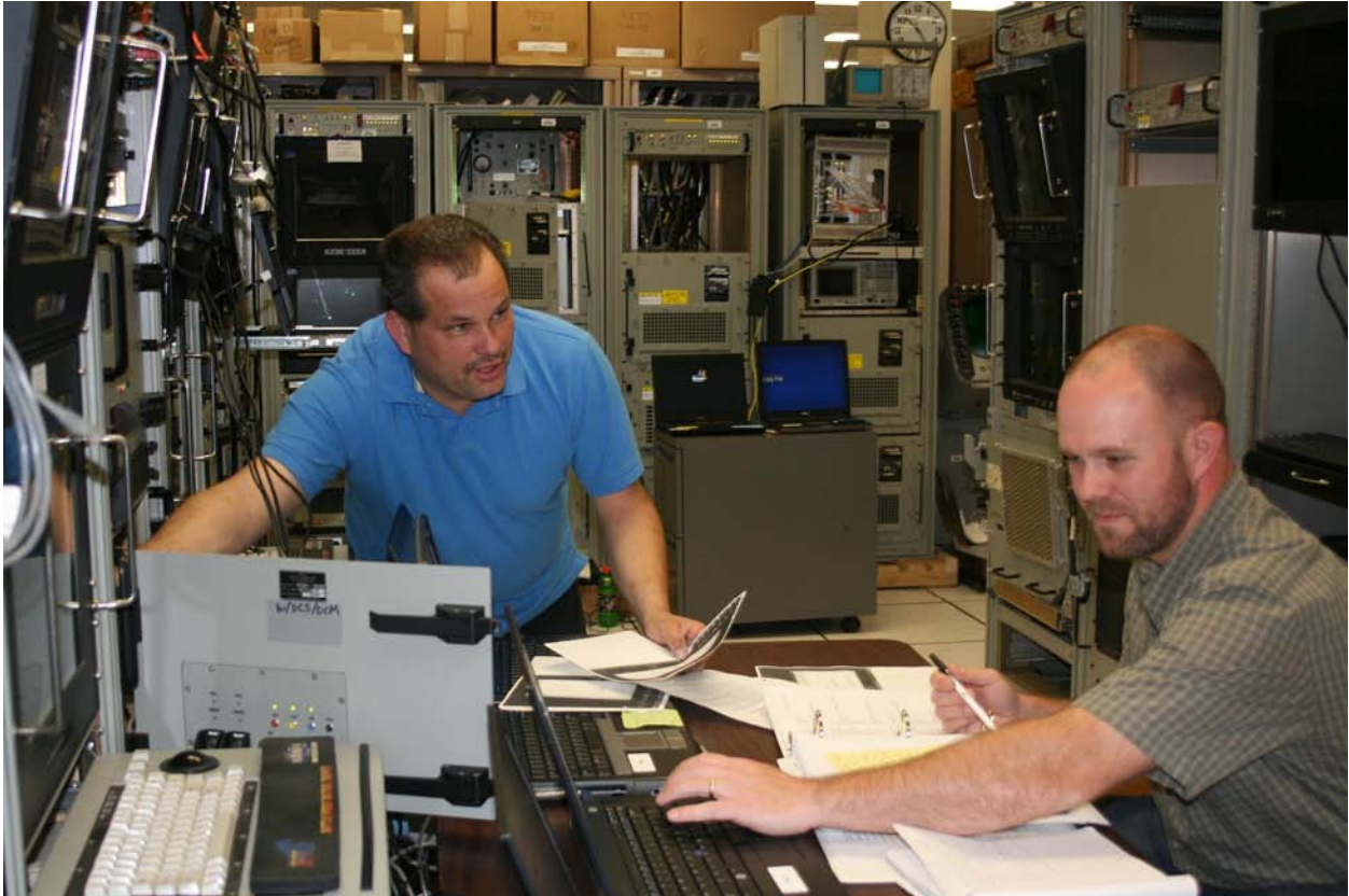
Figure 6. From left, Electronics Technicians Randy Constant and Steve Farmer conduct single board computer testing in the Integrated Training Systems Lab Complex at CDSA Dam Neck to determine the reuse viability of recovered parts, in support of the BFTT ISEA design teams recycling and refurbishing efforts.
