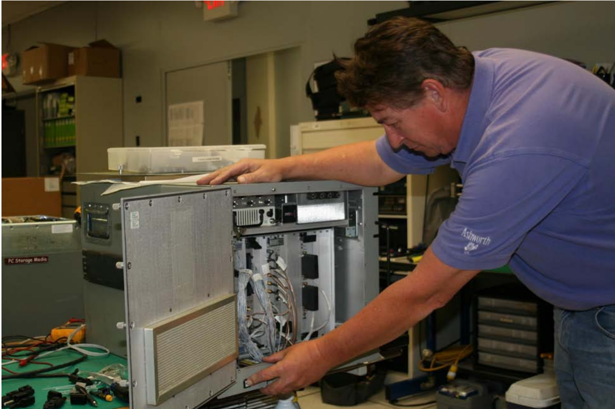
Figure 5. Electronics Technician, Mike Ellis refurbishing the Trainer Stimulator Simulator System is support of the BFTT ISEA design teams efforts to incorporate Removal of Hazardous Substances (RoHS) into both obsolescence mitigation and new design efforts for hardware.
