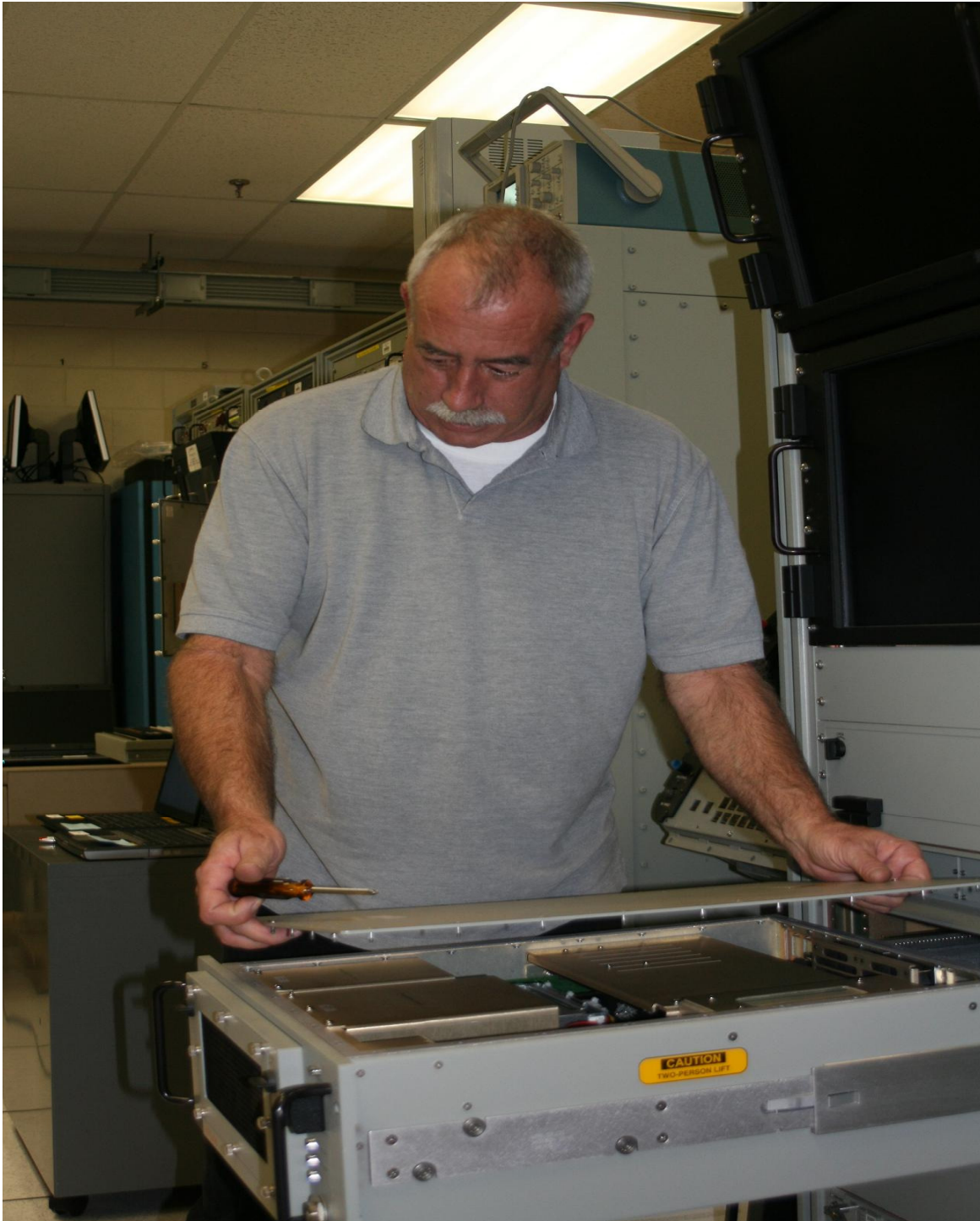
Figure 1. Mark Schroeder, BFTT ISEA design team member, removes the cover from the BFTT Operator Processing Console (BOPC) Advanced Technical Extended (ATX) chassis. The COTS motherboard computer enclosed within the chassis was a RoHS hardware replacement component.
