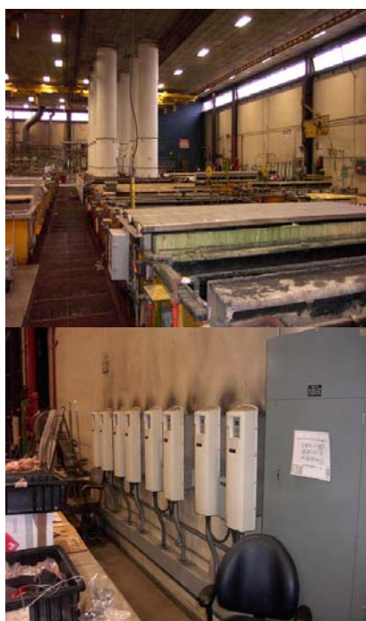
Figure 5 – New Exhaust Stacks Cover (top) and Programmable Direct position Digital Control Panels (bottom)
