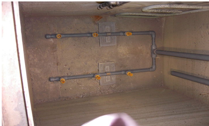
Figure 4 – New Mixing System Eductors Installed in an Empty Plating Tank
