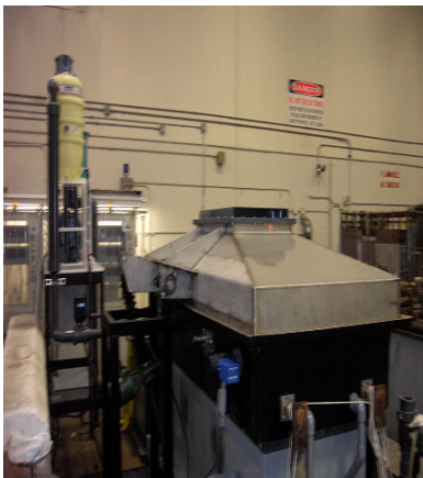
Figure 3 – New Chrome Cover with Exhaust System Left in Photo
