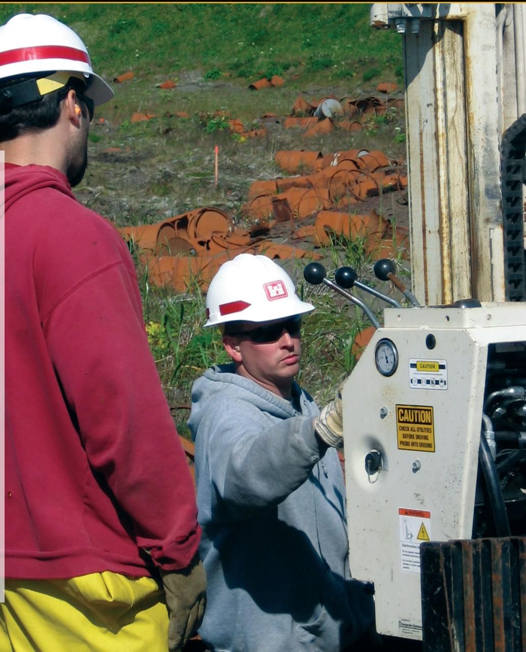
On this page: Will Mangano (left) and Jacob Sweet (right), USACE-AK, operate the Ultra-Violet Optical Screening Tool (UVOST®) and Geoprobe™ drill rig on Tanaga Island. (USACE photo)
