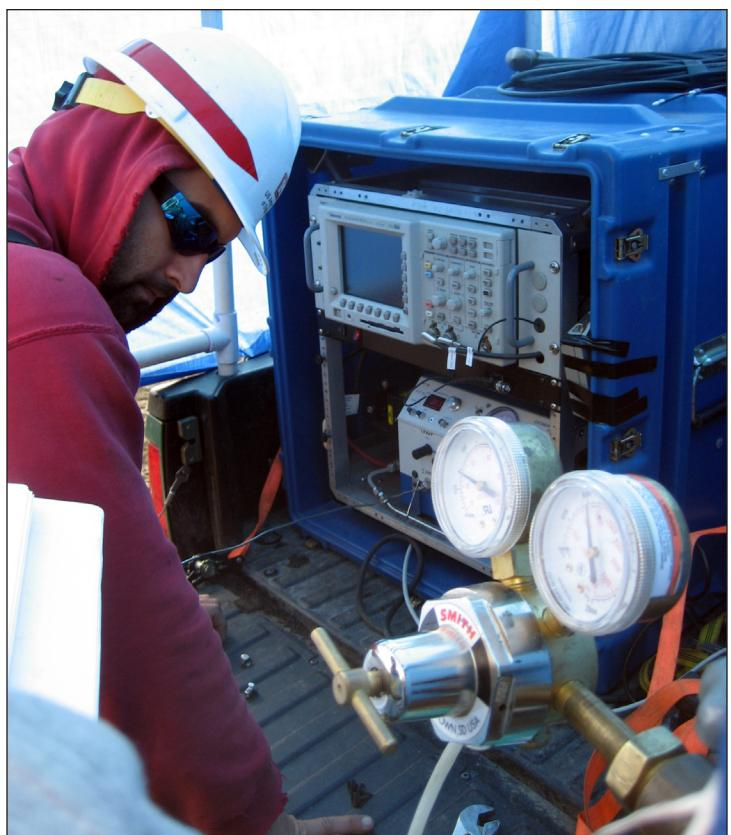
Will Mangano, USACE, operating the UVOST® innovative technology. Laser-induced fluorescence is detected by the oscilloscope, which then displays the results on a nearby computer screen in real-time.
