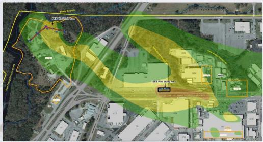
Two separate Pilot Studies were required for the validation of Innovative Technologies in the two treatment zones. The ISEB Pilot Study addresses the high concentration Near-Source Zone 1 and the PRB Pilot Study addresses the lower concentration Downgradient Zone 2.
