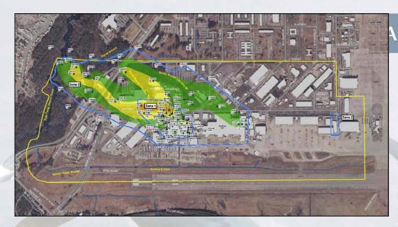
Contaminant Concentration Map illustrating the Central Groundwater Plume and it's relation to Operable Unit 1, as well as the delineation of the two separate treatment zones.
