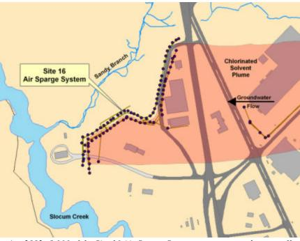
During 2002, O&M of the Site 16 Air Sparge System was contracted to a small business at a savings of more than \$21,000. The Air Station implemented air sparging at Site 16 as an interim measure to prevent groundwater contaminants from migrating to the environmentally sensitive Sandy Branch and Slocum Creek.
