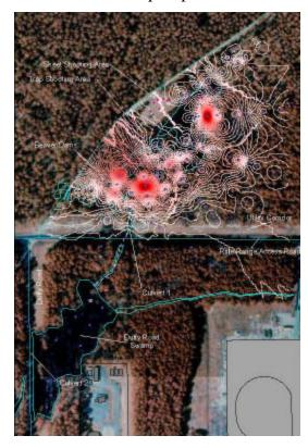
Lead concentration contours depict expected shotfall pattern and demonstrates site hydrology resulted in lead transport downgradient toward beaver dams into low energy forested wetland.
