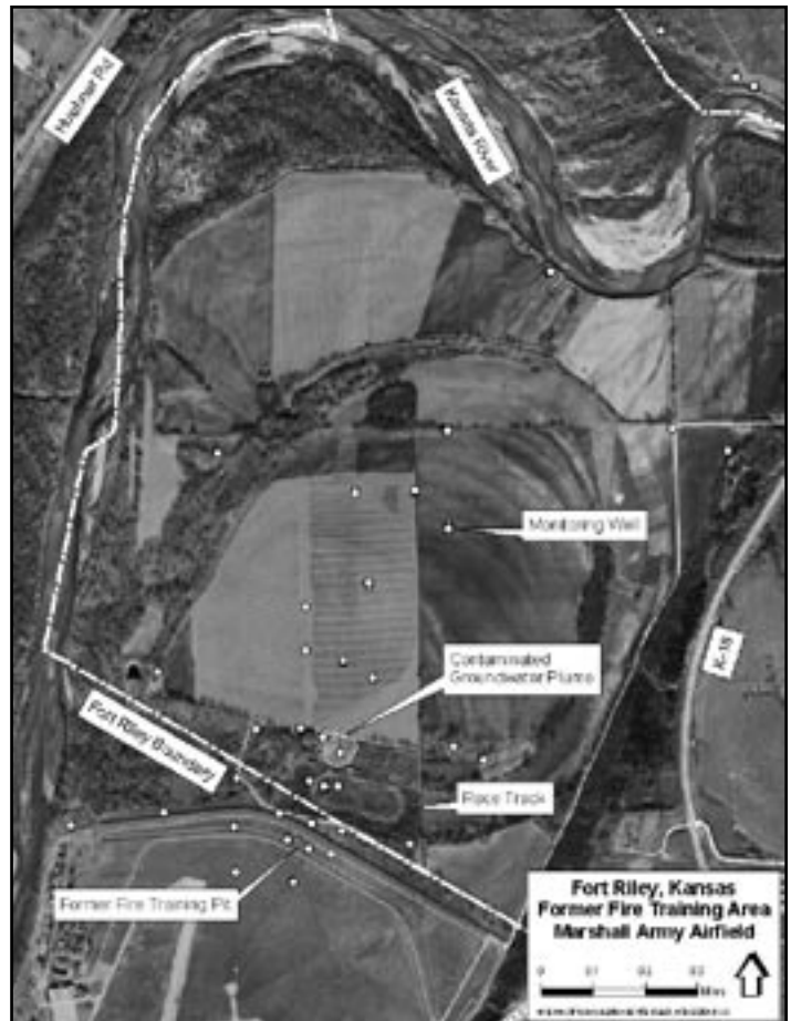
▲ This map shows the former fire-training area where Fort Riley has conducted soil vapor extraction bioventing to treat contamination.
