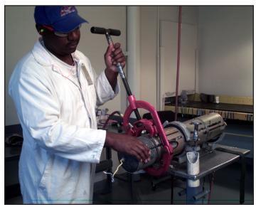
▲ An employee at the Missile Recycling Center removes the TOW missile flight motor during the disassembly process.
