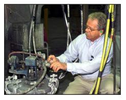
A technician checks the pot pressures on painting equipment.
