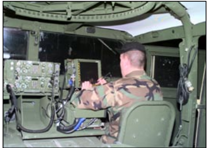
▲ The Blue Force Tracking System, shown above, helps the war fighter to pinpoint the vehicle’s location and improve situational awareness. TYAD personnel fabricate BFT installation kits and have integrated the systems into thousands of Army vehicles.
