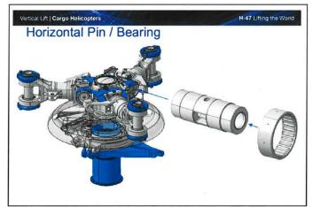
CH-47F Block II IRS Horizontal Pin.
