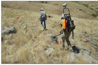
Field crews use the "Parsons Digital Mapper." The hand-held digital geophysical mapping (DGM) device allowed uxo technicians to perform DGM surveys in rugged terrain and with high magnetic interference. Rocky terrain and slopes are representative of the site.
