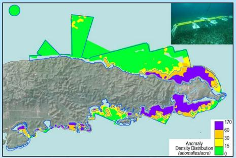
Figure 11. Distribution and density of potential munitions on and beneath the seafloor identified by the towed magnetometer array.
