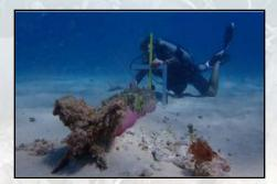
Figure 10. Diver measuring the movement and burial of a munitions surrogate.
