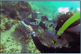
Figure 8. POCIS and grab water sample collection adjacent to an underwater munition.
