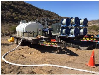
Vandenberg AFB developed mobile in-situ remediation equipment using groundwater recirculation. The equipment helps to implement a sustainable approach to efficiently remediate a wide array of sites while also saving water.
