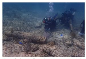
Scientific divers collect sediment pore water samples adjacent to an underwater munition. Staff collected pore water, grab surface water, and sediment samples to help evaluate Polar Organic Chemical Integrative Sampler (POCIS) data. The POCIS technology helped demonstrate munitions constituents are not a significant concern in the marine environment, which may save millions of dollars at Vieques and other sites.
