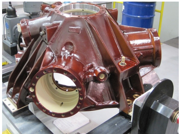
The CRH Program ESOH Team identified and eliminated hazardous materials used during CRH assembly. Efforts reduced HAZMAT exposure for operators and maintenance personnel and doubled the coating life, thereby reducing lifecycle sustainment costs.
