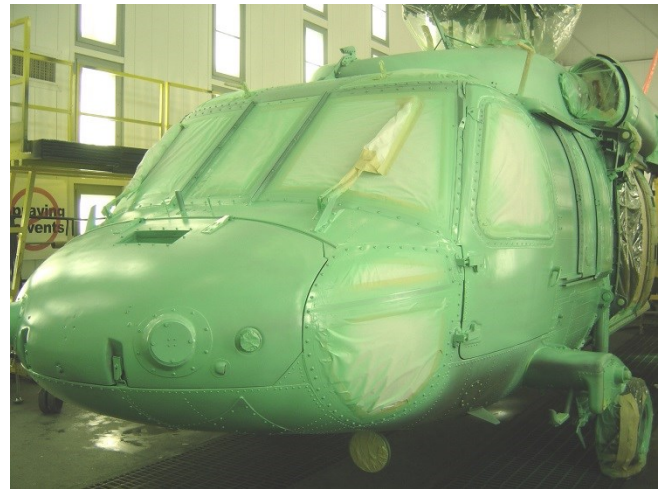
Hazardous hexavalent chromium (Cr6+) primer on the interior and exterior of aircraft have been replaced with non-chrome alternatives through targeted identification and risk mitigation processes. Replacements eliminate exposure risks for operators and maintenance personnel.
