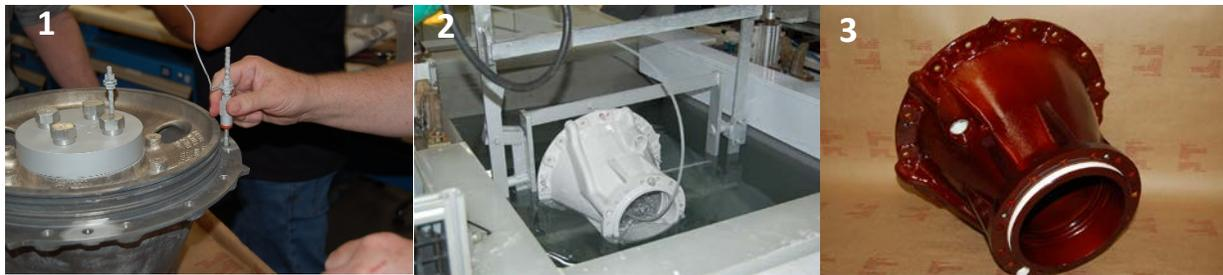
**Figure 2:** As part of the ESTCP Demonstration, a UH-60 Output Housing is masked (1), Tagnite anodized (2), sealed with Rockhard.
