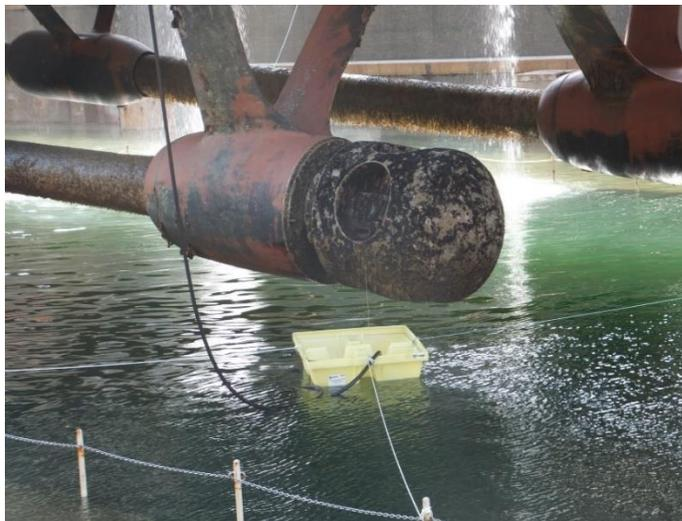
170617-N-YU361-036 SRF-JRMC oil spill management team members tethered a floating oil containment pallet in position beneath the damaged propulsion hub of USS ANTIETAM (CG 54) in dry dock No. 5.
