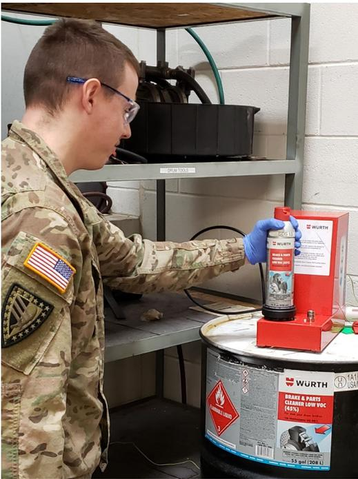
An employee demonstrating the refilling process. The process recharges the can without taking more than a couple minutes from the employee's day. It is simple enough to only require one person and minimal personal protection equipment.
