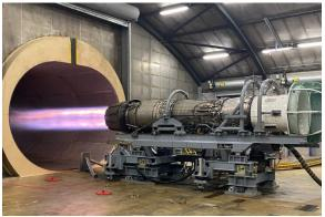
Jet Engine in Afterburner Mode
