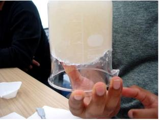
EF Polymer blended with water, showing its water retention capacity.
