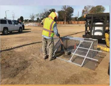
The Naval Base Ventura County (NBVC) Environmental Restoration Program (ERP) developed an innovative mobile chemical agent containment hood to remediate chemical agent identification sets containing phosgene, chloropicrin, mustard gas, and lewisite.
