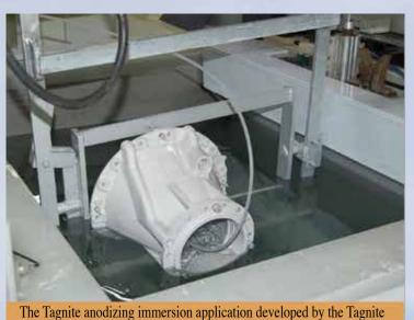
Technical Working Group (WG) reduces exposure to carcinogenic hexavalent chromium. The capability extends the life of magnesium components and alleviates regulatory challenges.
