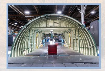
Interior of a production C-130J with new nonhex chrome finish. Eliminating hex-chrome from C-130J interior finishes can cut over 2,100 pounds of hex-chrome per year; reduce hazardous material issues with life-cycle/maintenance of aircraft painting; and limit employee carcinogen exposure.
