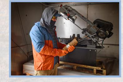
Ordnance and Explosive Safety Specialist Mr. James Ennis prepares a 75 mm munitions debris item for cutting on a remotely operated bandsaw. Cutting a munition item helps render it safe by allowing observers to confirm that the item is empty and no longer intact.
