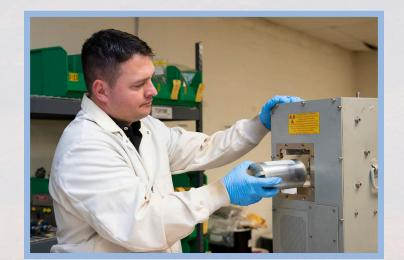
Mr. Seth Walton disassembles a Navy Shipboard Chemical Agent Detector Alarm. AFRRAD provided the Navy with a radioactive material (RAM) recycling outlet for chemical agent detection alarms, which cut waste volumes by over 99 percent and enabled recycling of radioactive sources.
