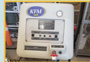
The KFM, LLC coolant purification system is used to recycle used antifreeze at Marine Corps Support Facility Blount Island. Shop personnel collect used antifreeze and transfer it into a tank. Once a sufficient volume is collected, it is processed through the system and transferred into a purified antifreeze tank for dispensing to shops.
