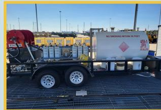
The Fuel Filtration Unit can process most off-spec fuel generated at Marine Corps Support Facility Blount Island. Shops collect off-spec fuel in intermediate bulk container totes labeled "Off-Spec JP-5 Fuel for Recycling," which are visible in the background.
