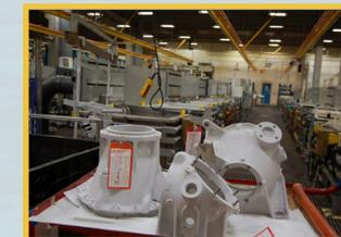
Three magnesium housings coated with Tagnite. Tagnite is an alternative pretreatment to the legacy Cr6+ conversion coatings. It is not only a safer alternative but it also provides superior corrosion protection over the legacy process.
