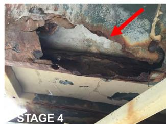
Examples of corrosion during ground vehicle parts inspections. The U.S. Army Combat Capabilities and Development Command researching Cr6+ ground vehicle product alternatives must work closely with the corrosion office to ensure proposed replacement products effectively protect the equipment and soldiers in all environments.
