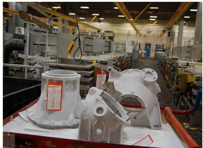
Three magnesium housings coated with Tagnite. Tagnite is an alternative pretreatment to the legacy Cr6+ conversion coatings. It is not only a safer alternative but it also provides superior corrosion protection over the legacy process.
