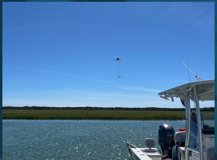
The aerial drone equipped with a magnetometer to identify subsurface anomalies in an inaccessible area.
