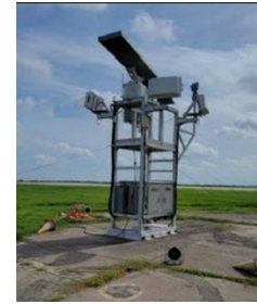
Photo 6: A fixed Doppler radar system provides 24-hour monitoring of avian movement within a 4-mile radius of the airfield.
