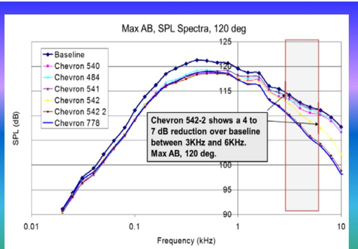
**Figure 5: F/A-18 Jet Noise Reduction - Chevron Nozzle Static F404 Engine Test**
