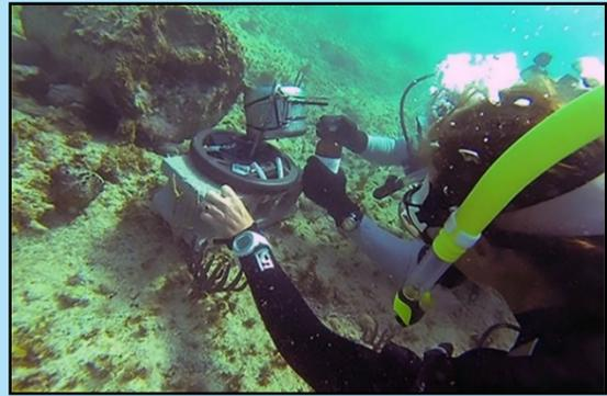
Figure 8. POCIS and grab water sample collection adjacent to an underwater munition.
