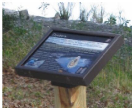
Digital files for the signs were then embedded in weather-resistant fiberglass resin. Metal frames conforming to NPS outdoor sign standards were chosen to support the signs, and special tamper-resistant screws mount them to
