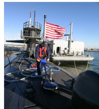
*High Pressure Jet Blasting on anti-skid from submarines*
