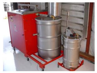
Cleaner to be used again. The residue, consisting of paint solids, is a fraction of the original waste thinner volume which saves on thinner costs, waste costs, and significant waste minimization is achieved. At the current waste paint sludge generation rate by DnyCorp, the Air Station will save approximately \$26,920 per year in sludge disposal and virgin solvent purchases.
