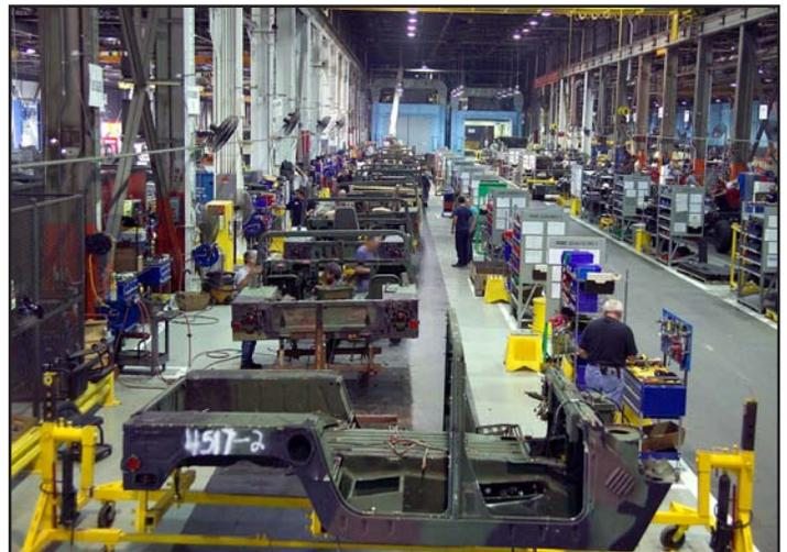
*HMMWV's are disassembled upon arrival at Letterkenny to prepare them for repair and maintenance prior to repainting.*
