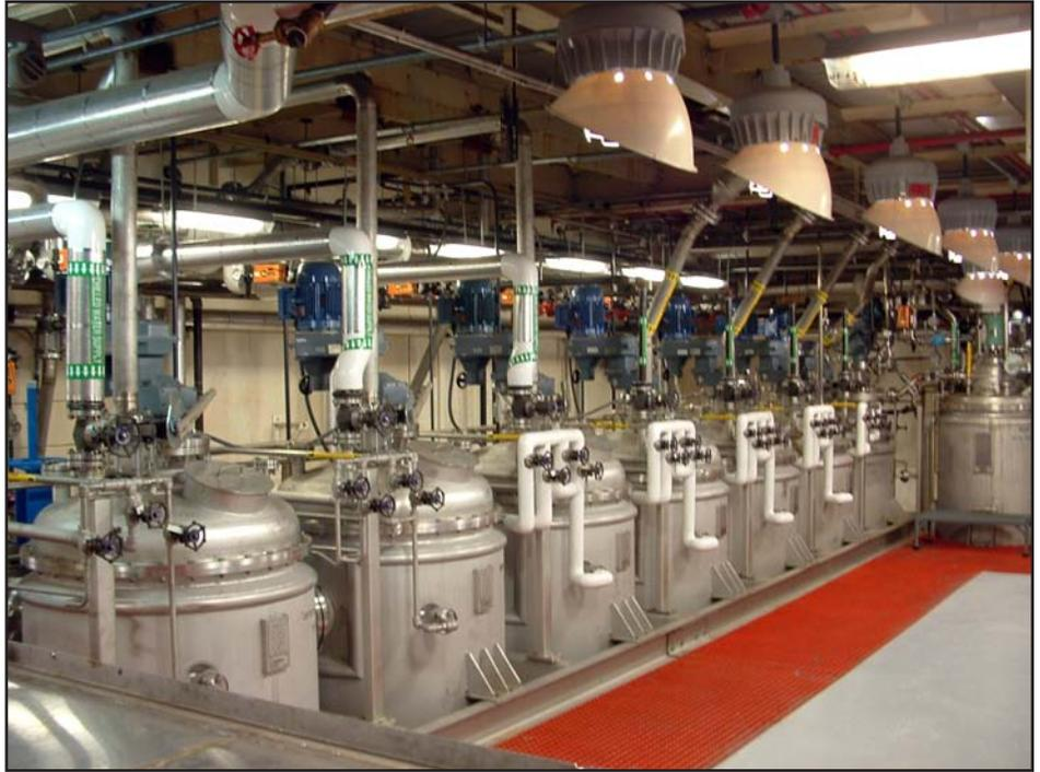
*TNT weak nitric acid crystallizer vessels eliminate the generation of hazardous red water.*
